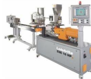
Compounding reactive extrusion (10 kg/h)
