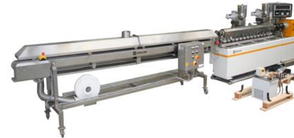
Compounding reactive extrusion (30 kg/h)
