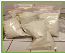
grounded PIR foam at Materia Nova
